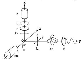
Fig. 1. A schematic drawing of the excitation-detection configuration. EG: electron gun; D: detector; FR: Fresnel rhomb prism; L: lens; N: nozzle; P: polarizer.
